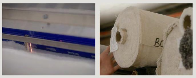
Materials Reuse – Dacron All Dacron off-cuts are recycled and sent back to the manufacturer, re-teased and made into new Dacron.
